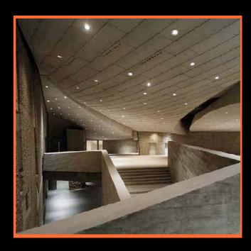
Magma's column-free, 30,000 square-foot main lobby is wide, deep and dark, and opens to the expansive main hall where the high, fibre-cement ceilings part to allow natural light. Retaining walls surround the complex and guide visitors to the forecourt of the building. A concrete bridge extends from the upper level as a secondary entrance on the sloping site.
