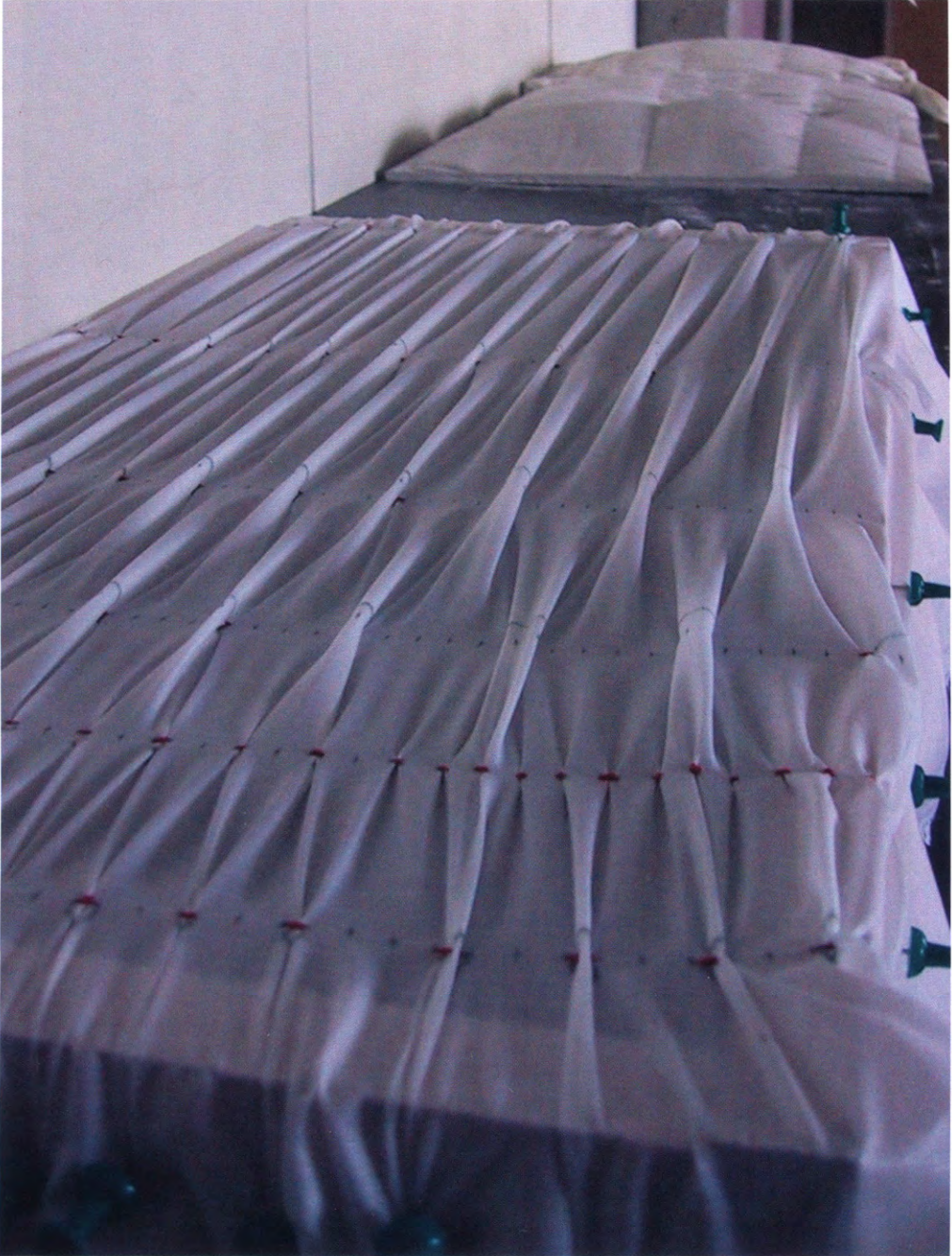
Fabric formwork, Smocking v5 (Courtesy Kentaro Tsubaki)
