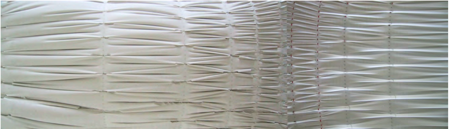
Smocking V5: Composite image of the plaster cast and fabric formwork. Photo: Tsubaki©
